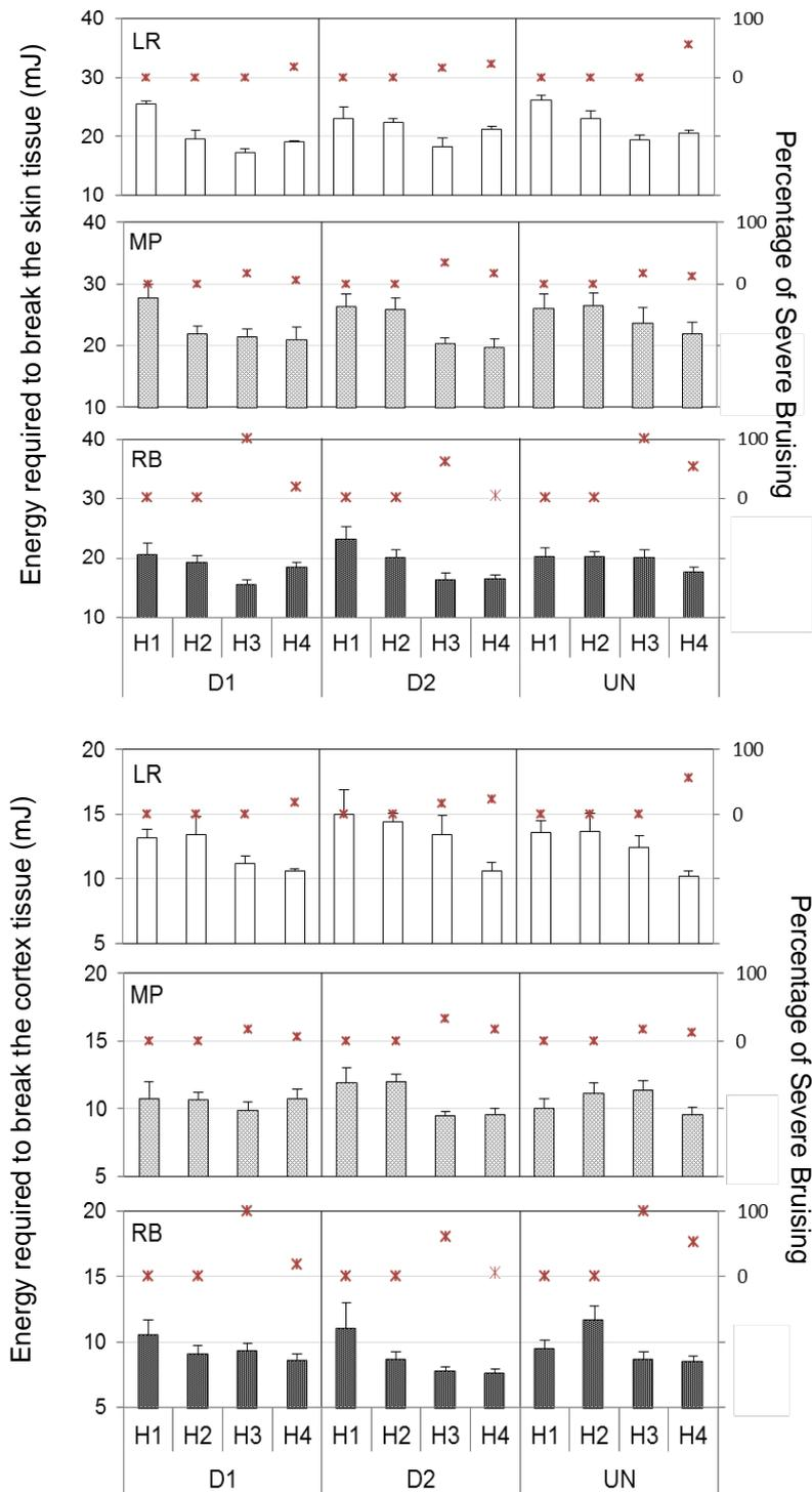
Figure 4.2 Effect of variety, harvest time and defoliation regime on energy to break the cortex tissue in mJ (bars) and percentage of severe bruising (scatter) from crops harvested in early August (H1), late August (H2), early September (H3) and late September (H4), defoliated early August (D1), late August (D2) and undefoliated (UN), field trial 1. Values bars show mean (n=9), errors bars are SE and scatter shows incidence (H1-H3 n=9, H4 n=18).
